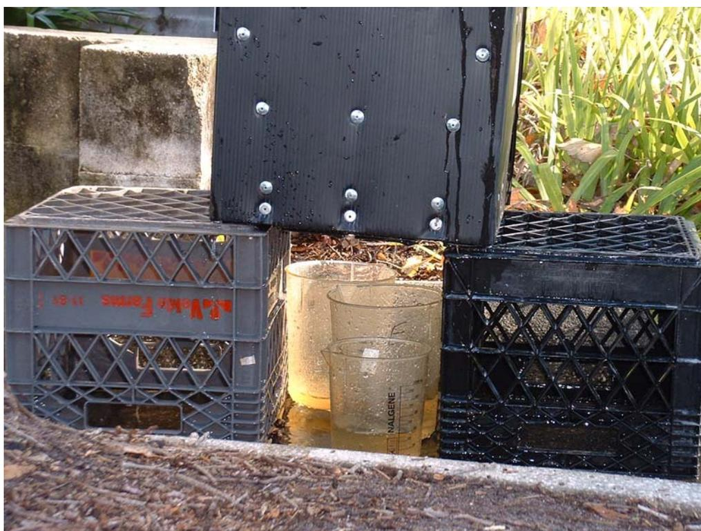
Figure 3-12. Collection of Outflow Samples for the Ultra-Urban Filter.
