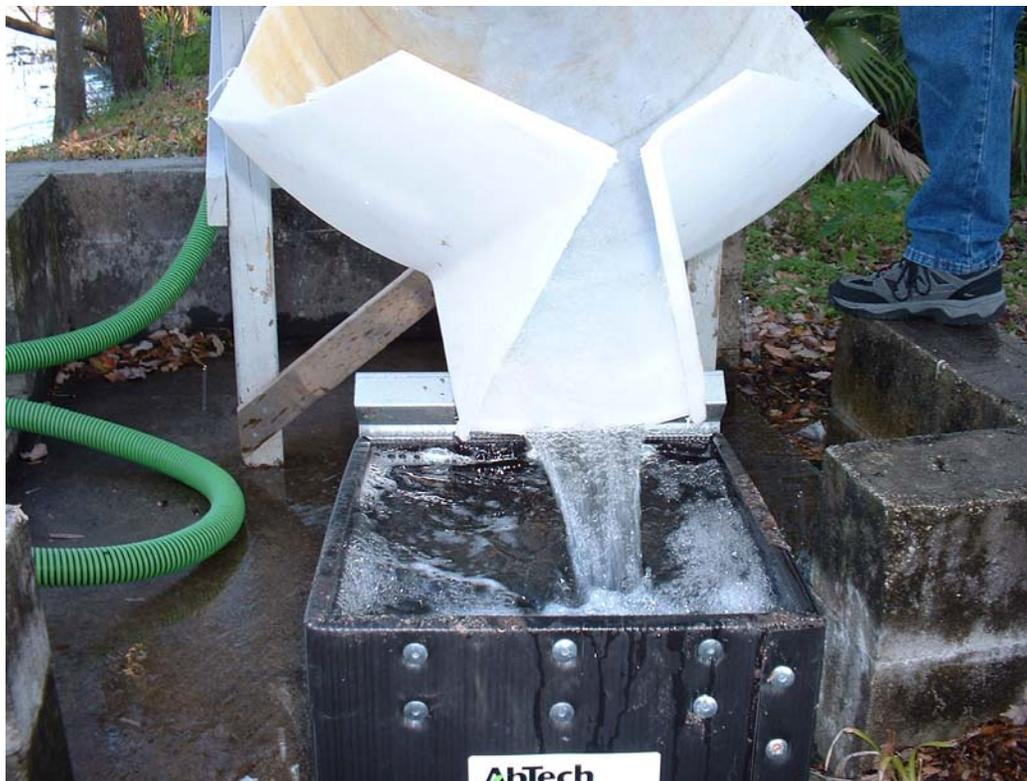
Figure 3-10. Hydraulic Performance Testing Using the Ultra-Urban Filter.
