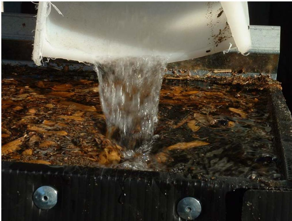
Figure 4-14. Loss of Leaves During Overflow of the Ultra-Urban Filter Unit.
