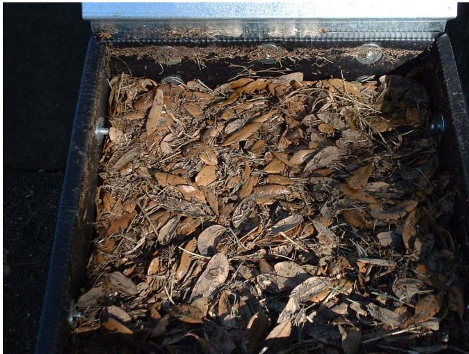
Figure 4-12. Accumulated Solids in the Ultra-Urban Filter Unit.
