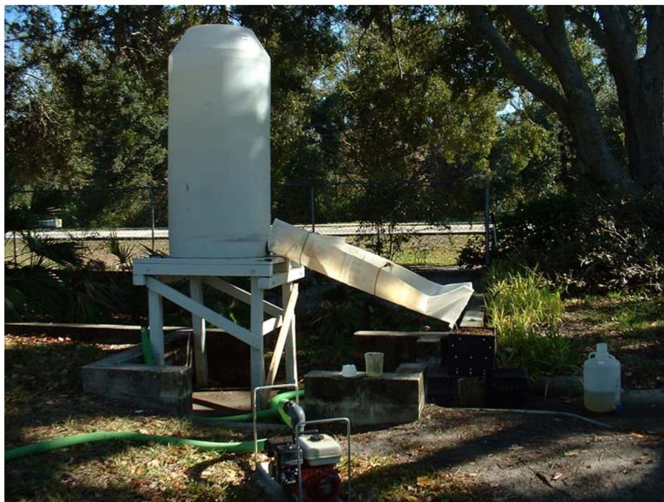
Figure 3-7. Pilot Testing Apparatus for the Hydro-Kleen and Ultra-Urban Filters.
